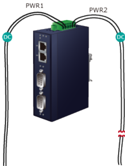
DC/DC Power Failure
