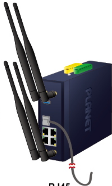
RJ45 Connection Link Down
